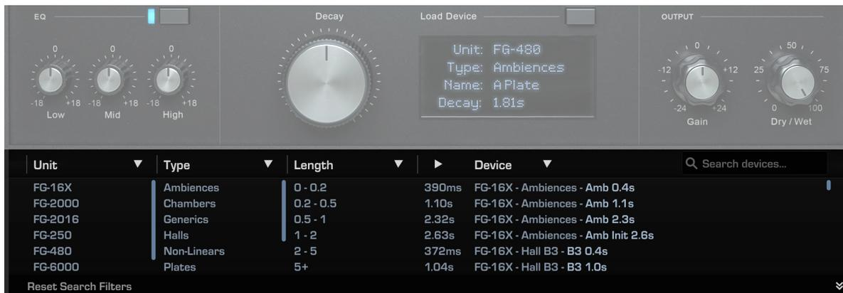
The Device Browser is a quick search tool that helps to narrow down the devices by reverb unit, type of reverb, and reverb length.
